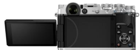
Swivelling high resolution touchscreen LCD
